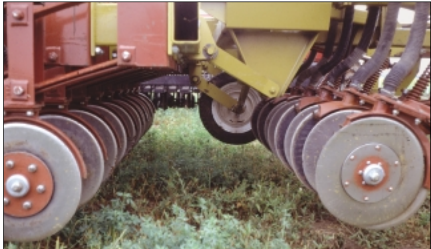
A no-till planter showing seed openers and steel press wheels.
